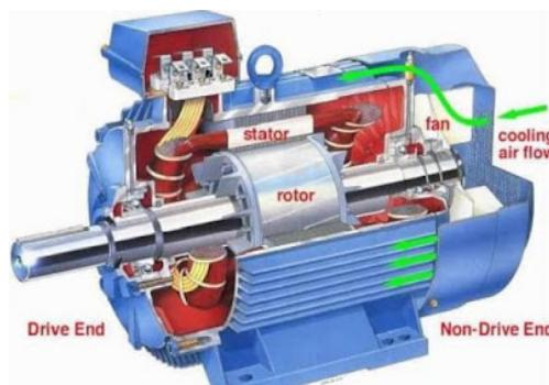
This three-phase motor operates on a fundamental premise. A spinning magnetic field will be produced at a specific speed when the stator coil is subjected to a three-phase voltage source. The equation  $N_s = 120 f / P$  can be used to calculate the speed.  $N_s$  stands for speed,  $f$  for source frequency, and  $P$  for the motor's magnetic pole.
